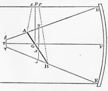
$G\pi$  may bee equal to Gp; erect  $\pi\sigma$  &  $\pi\tau$  equal to ps & pt, & from  $\sigma$  &  $\tau$  draw two times,  $\sigma D$  &  $\tau E$ , to the utmost parts of the concave, whin the Tube intersecting AB in A & B; & AB shall bee the long diameter of the ovall; which bisect in x, & perpendicular to Fx erect xy & xz occurring with  $\sigma D$
